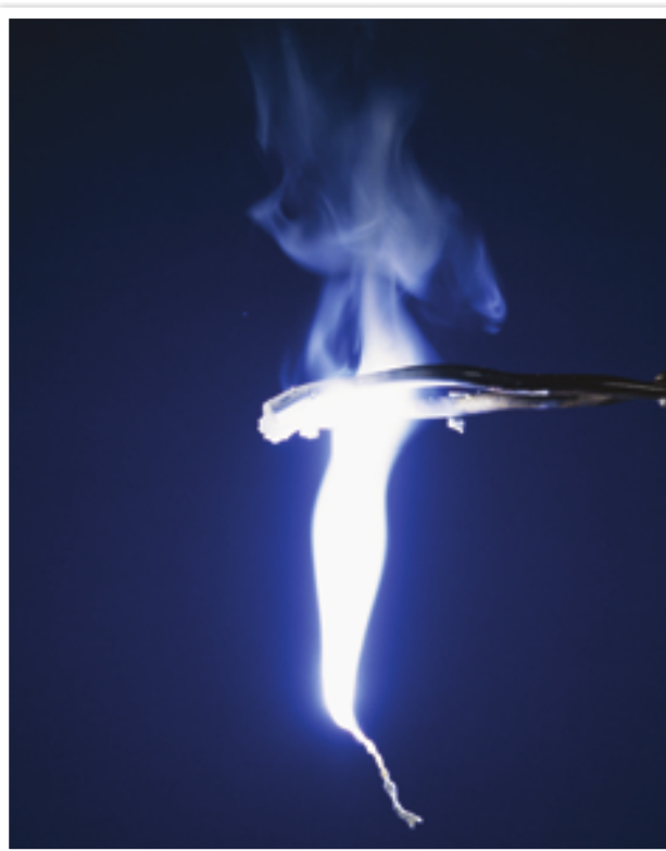
Fig 3.2.4 Magnesium burns in oxygen and releases intense light that is dangerous to look at. This reaction is both a combustion reaction (involving oxygen) and a combination reaction (combining Mg and O 2 ).
