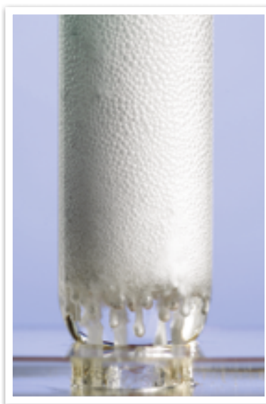
Fig 3.1.6 Bubbles in a liquid or solution are an indication that a chemical reaction is happening. Here hydrogen gas is bubbling out of a reaction between magnesium metal and hydrochloric acid.
