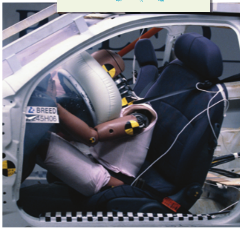
Fig 3.2.6 The deployment of an airbag during a crash is caused by a decomposition reaction.
